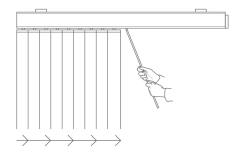
If any of the slats are out of alignment, twist the wand control until the slats are in the closed position, then continue to twist the wand until all the slats are fully aligned.
