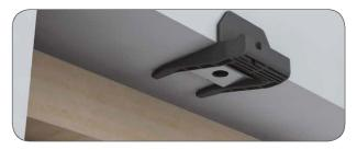
2. Take the tool and bracket to the window recess. Butt the flat vertical face of the tool against the outer face, and hold the bracket against the top face of the recess approximately 100mm in from either side of the recess.
