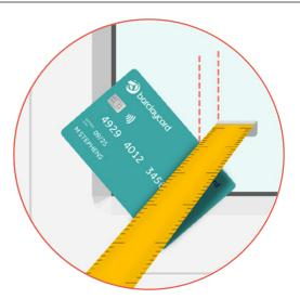
Using a bank card or something similar, place it flat on the frame corner. Using your tape, measure the depth between the glass and the card. This will give you your bracket size.
