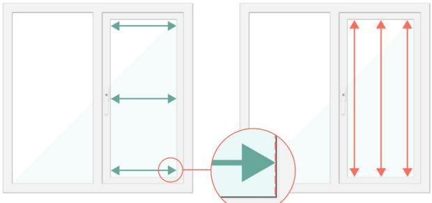
Only measure the visible glass, do not include any beading or seals. Measure from inside the frame where the glass meets the seal/beading. Measure every window and door, don't assume that they are the same sizes.
