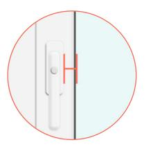
The edge of any handles or ventilation units must be more than 25mm away from the edge of the glass.
