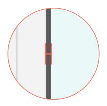
The width of the seal/beading must not exceed 6mm.
