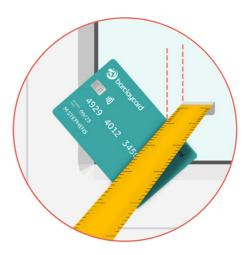
Using a bank card or something similarly flat, place it flat against the front corner of your window/door frame. Using your tape, measure the depth between the glass and the inside of the card.
